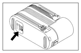
Your tire sealant and compressor kit has an accessory adapter located in a compartment on the bottom of its housing that may be used to inflate air mattresses, balls, etc.
